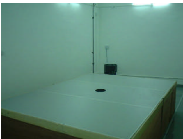
Set-up of Metal Ceiling System (Type E-600 & Type E-200) in the Reverberation Chamber
